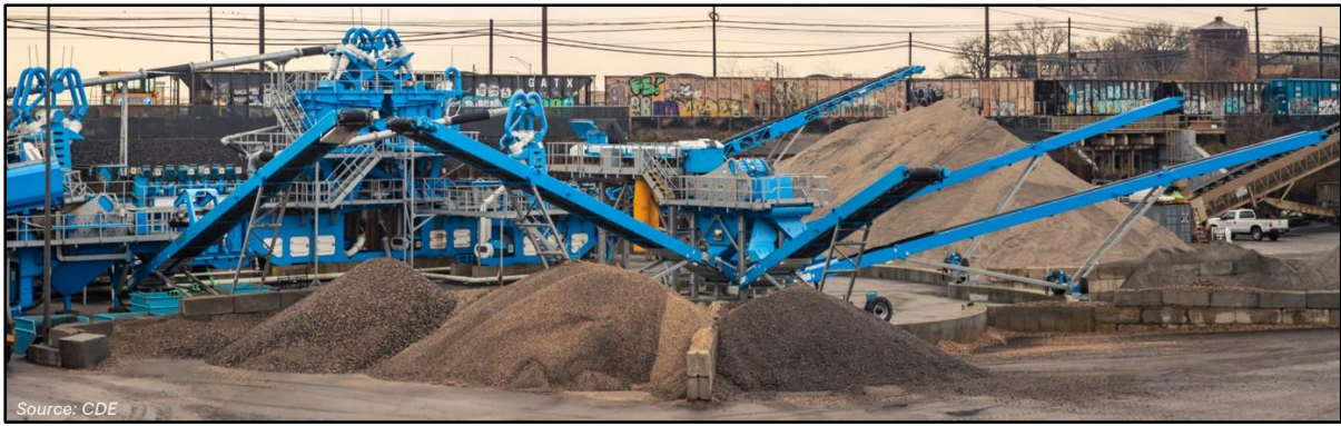
Figure 7: Image of a mobile soil washing plant removing contaminants from soil, to facilitate its reuse on site (photo from CDE, n.d.).
